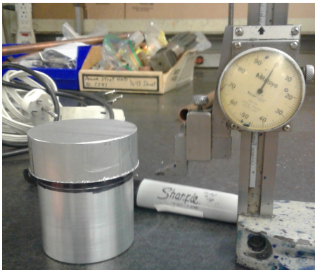
Figure 1: Marking the 'no-go' line using the height gauge. Measure 0 from the flat table, and account for facing the end of the part and the bandsaw blade width for cutting off excess.
