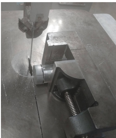
Figure 3: Cutting off the excess in the bandsaw. Using a vise to grip the part is recommended.
