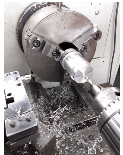
Figure 2: A turned-out part on the 3-jaw lathe. You can ignore the drill bit, drill chuck, and the hole in the part; these were made by mistake.
